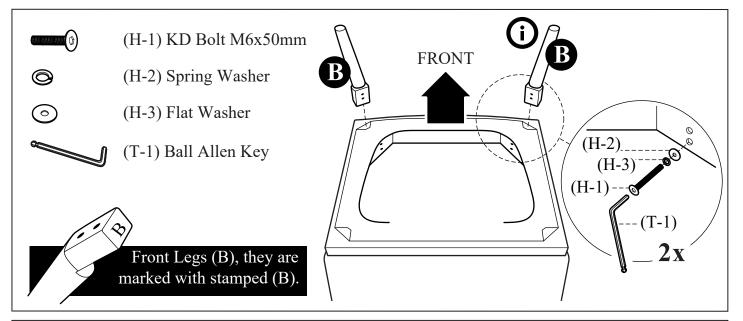
Align and insert Front Legs (B) into position as shown in the diagram above. Secure both legs using KD Bolts M6x50mm (H-1), Spring Washers (H-3) and Flat Washers (H-2) stacking the hardware in the order as shown. Fully engage bolts but do not tighten them until Step 3.
