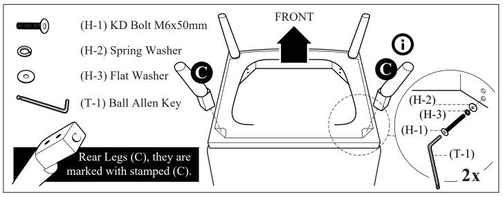
Align and insert Rear Legs (C) into position as shown in the diagram above. Secure both legs using KD Bolts M6x50mm (H-1), Spring Washers (H-3) and Flat Washers (H-2) stacking the hardware in the order as shown. Fully tighten all bolts from this and the previous steps.
